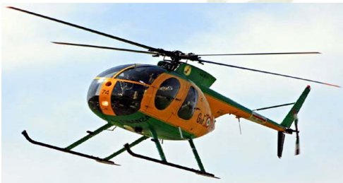
25 Helicopters OH 500 Max speed 130/156 knots Endurance 2,5 hours
