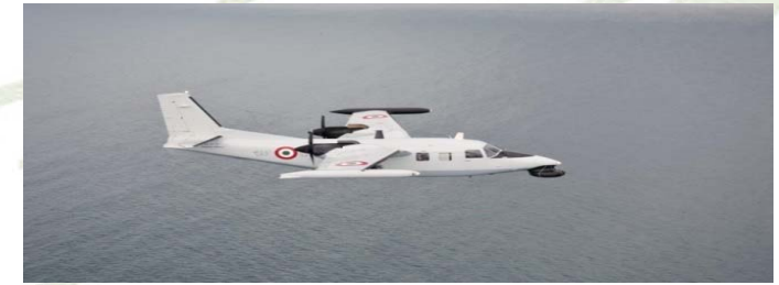
6 Aircraft P 166 DP 1 Max speed 220 knots Endurance 5 hours
