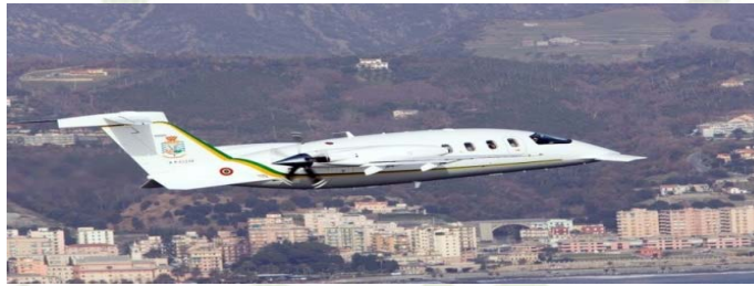
2 Aircraft P 180 Max speed 260 knots Endurance 4 hours
