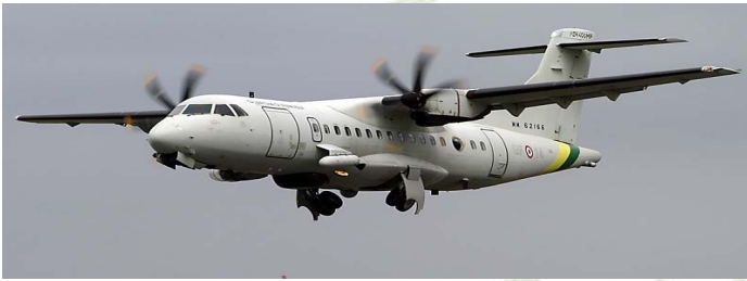
4 Aircraft ATR 42 MP Max speed 250 knots Endurance 8 hours
