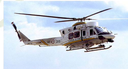
16 Helicopters AB 412 HP Max speed 140 knots Endurance 4 hours
