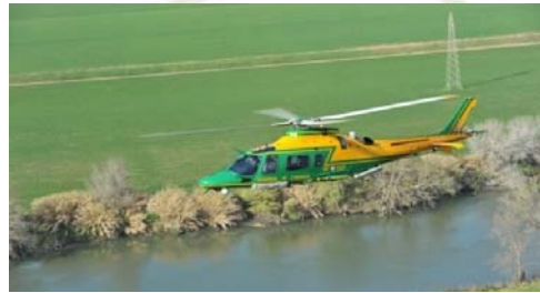
17 Helicopters A 109 N Max speed 153/168 knots Endurance 3/3,5 hours
